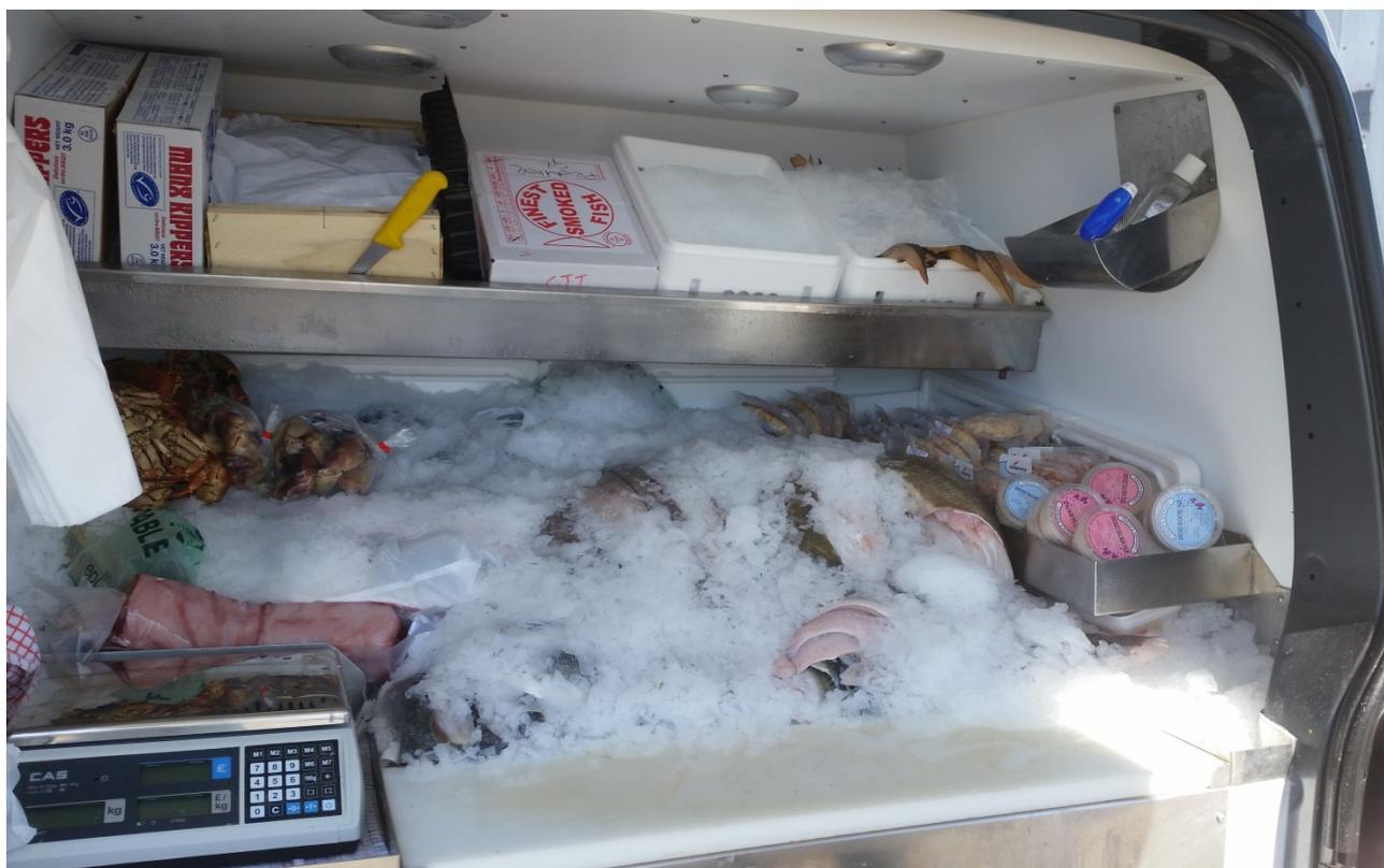
The selling area invariably will comprise a tank to contain ice within which the chilled fish is stored. The ice tank may have a surround upon which a cutting board and scales are mounted, and which also provides useful storage space for knives, wrapping and items for sale.
